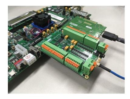
NeuralFMC is an FMC board with four ports of Intan RHD2000 series module. NeuralFMC is compliant with the VITA 57.1 standard and can be mounted on FMC (LPC and HPC) and FMC+ (HPC+).
