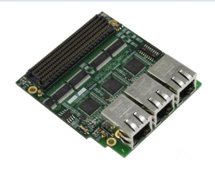
FMC-GbE-RJ45 is an FMC board with three ports of Gigabit Ethernet.
