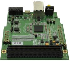
CON-FMC is a USB 3.0 FMC (FPGA Mezzanine Card) board which is compliant with the VITA 57.1-2010 standard. The CON-FMC provides USB 3.0 channel and can be connected to Windows/Linux/Android.
